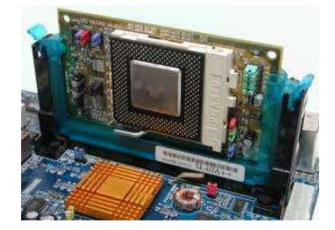
PGA (Pin Grid Array)
